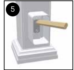
5 Remove rail and mark bracket flange holes.
