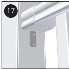
17 Seat balusters in to top rail. Snap/lock rail in place.
